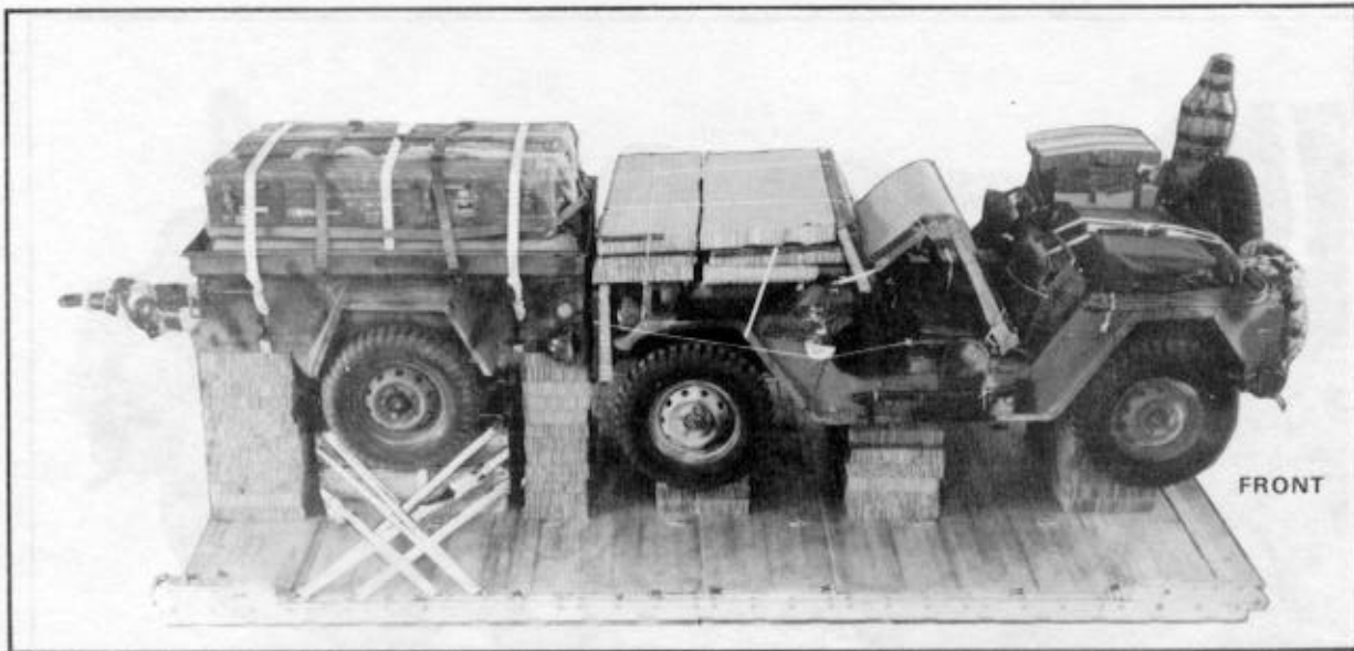
Figure 5-11. Truck and trailer set on platform
